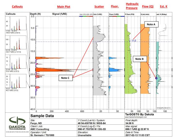
Estimated K: The estimated hydraulic conductivity (K) is internally calculated by utilizing pressure and flow data in conjunction with dissipation test(s) performed at each location. The estimated K is calculated by the equation:  $K = \ln(Q/P')*20.0 + 7.0$ .
