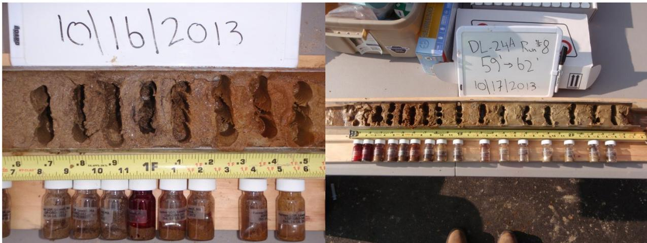
Figure 4. Cores sub-sampled at high resolution with ORO jars aligned with their content's origins.
