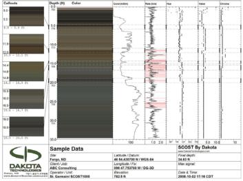
Dakota's SCOST system is more reliable and accurate than electrical conductivity and more cost effective than drilling. Another important benefit is the lack of investigation derived waste, as is the case with all of Dakota's optical screening tools.
