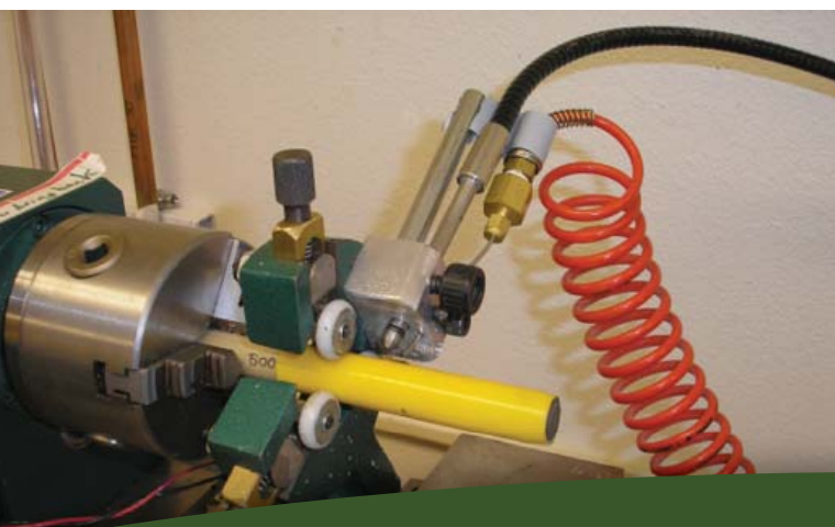
Dart logging system including lathe-based reader and UVOST system.
